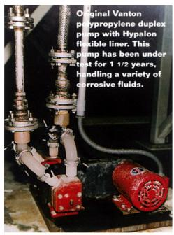
Original Vanton polypropylene duplex pump with Hypalon flexible liner. This pump has been under test for 1-½ years, handling a variety of corrosive fluids.
